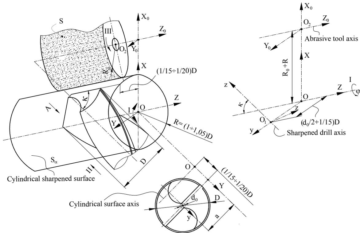
Fig. 1. Cylindrical sharpening of the straight edge drill: kinematics and reference systems
