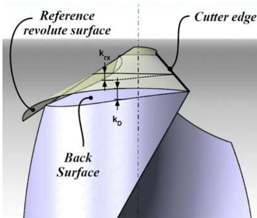
Fig. 6. Relieving values for the twist drill
