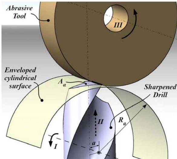
Fig. 5. 3D Models for the twist drill and for the main back surfaces
