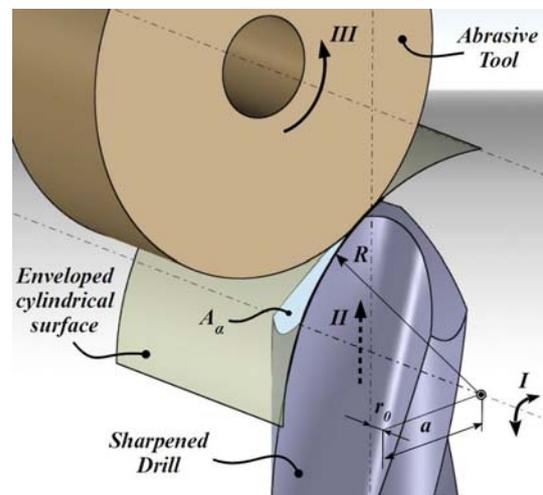
Fig. 8. Sharpening layout for the curved edge drill
