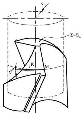
**Fig. 2.** The relieving size and the placing angle (on  $r_x$  radius cylinder)
