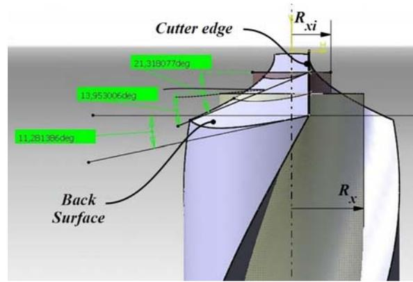
Fig. 7. Back angles along the main cutter edge
