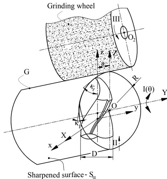
**Fig. 3.** Cylindrical sharpening of the curved edge drill: kinematics and reference systems
