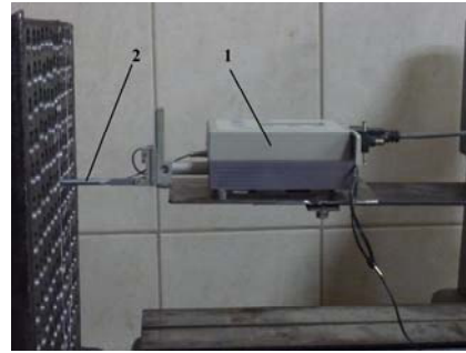
Fig. 7: Roughness measurement: (1) Taylor Hobson Surtronic 3+ Profilometer; (2) probe positioning
