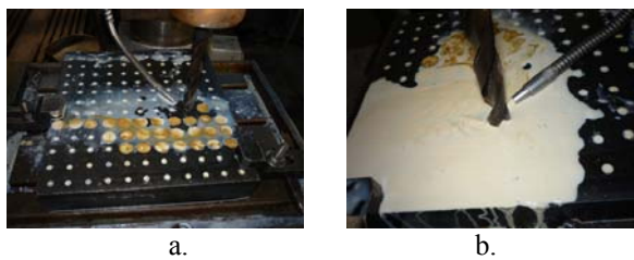
Fig. 6: Plate clamping system (a); Cooling system (b)
