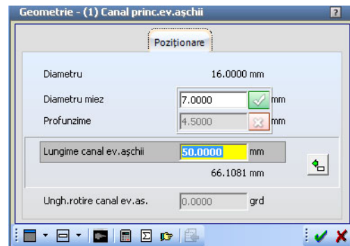
Fig. 26. Parameter values for the evacuation flute geometry
