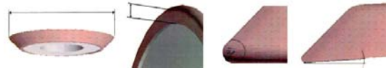
Fig. 32. The 11V9 Ø100 D64 disk: a) – diameter, b) – lateral width, c) – radius, d) – lateral angle
