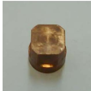
Fig. 7 The electrode with a negative form of the part
