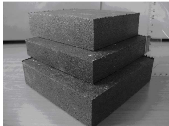
Fig. 8. Large and thick moulded rubber pads
