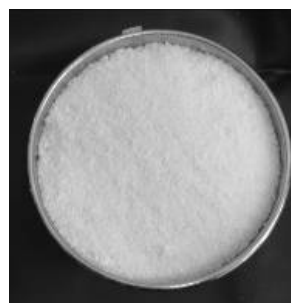
Fig. 2. Polyurethane comminuted powder
