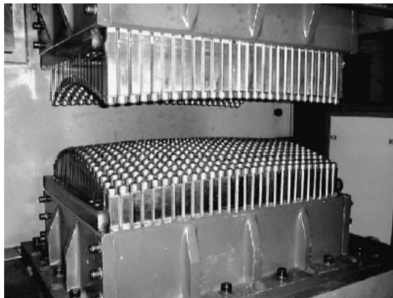
Fig. 8. Multipoint deformations die [24]
