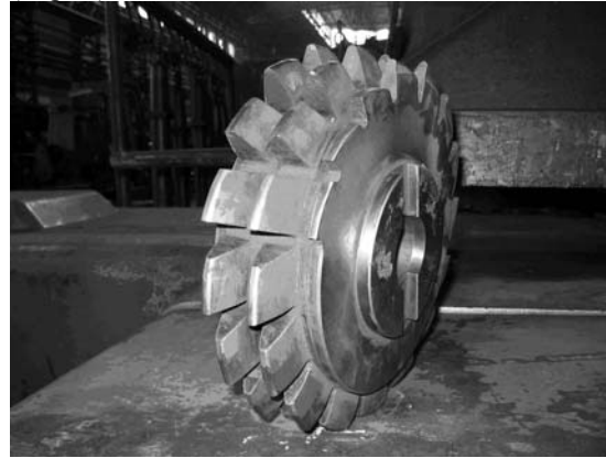
Fig. 2. Internal teeth profiled worm hob: m=10 ; z_2=95 ; x_2=0 .
