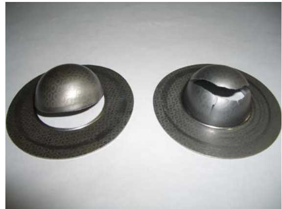
Fig. 6. - Failed specimen to the die edge to the left and a correct specimen on the right.
