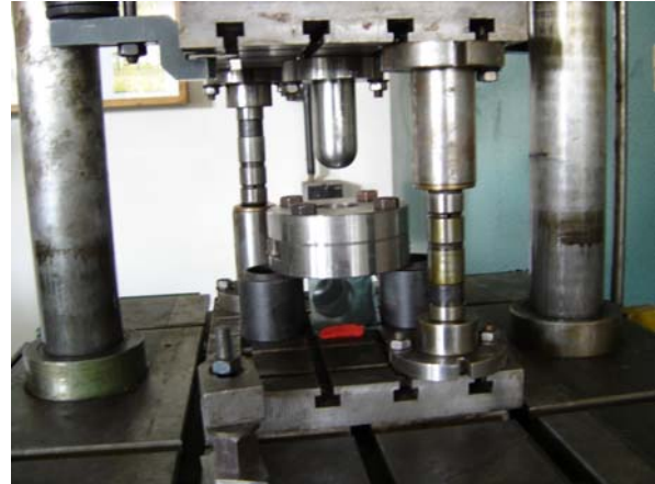
Fig. 2. - Tool arrangement and setup for Press 200 KN
