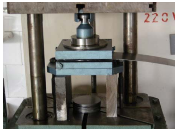
Fig. 3. - Tool arrangement for cutting
