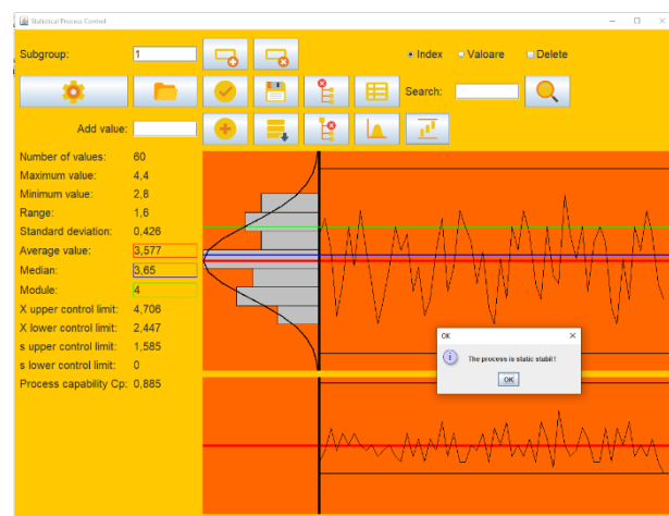
Fig. 18. Stability of the weld strength verification process: B2902 - B2704
