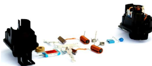
Fig. 2. Components of micro-motor flanges [17]
