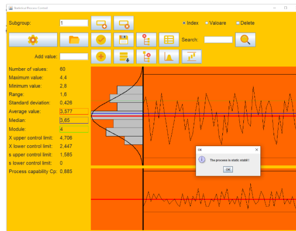
Fig. 17. Stability of the weld strength verification process: B2777 - B2704
