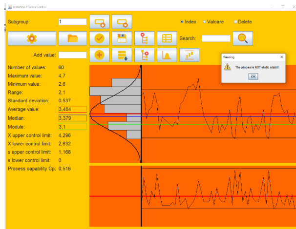
Fig. 20. Stability of the weld tensile/breakage verification process: B2902 - B2704
