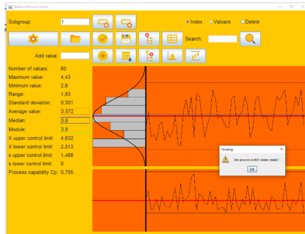
Fig. 19. Stability of the weld tensile/breakage verification process: B2777 - B2704
