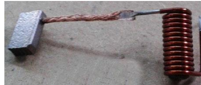
Fig. 7. Welding the collector brush wire to the impedance wire: 1 - collector brush wire; 2 - impedance coil; 3 - lower electrode
