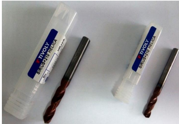
Fig. 6. Drills in the range of Ø8 and Ø10 mm diameters used in the processing of the plates
