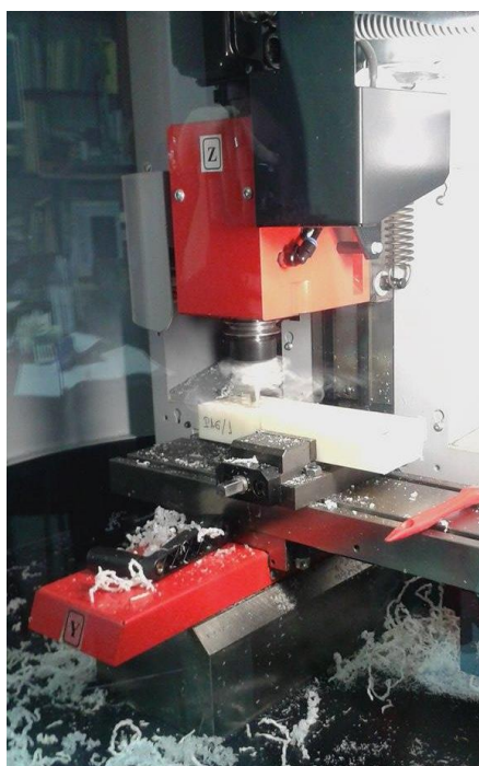
Fig. 7. The clamping system of the plate from EMCO MILL 55 CNC drilling machine
