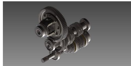
Fig. 22.5 speed synchromesh manual gearbox final assembly.
