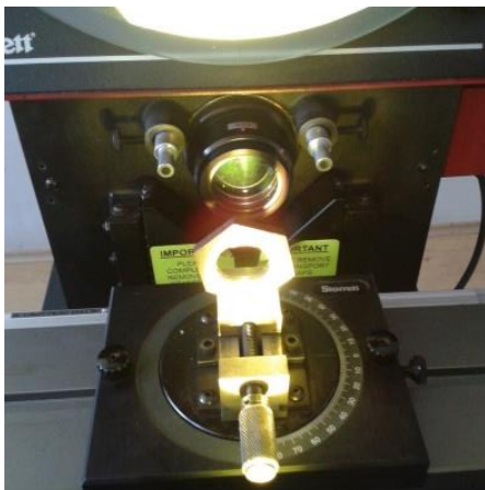
Fig. 1. Attach the part to the measuring device
